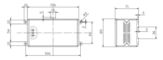
Figure 2.1 installation dimension of main engine
