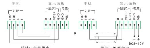
Fig. 4.11 Connection Method between Host and Display Panel
