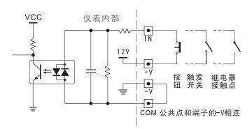
Figure 4.1 schematic diagram of switch input connection
