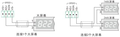
Figure 4.7 Schematic diagram of connection of large screen display Note: Two large screens can also be connected in parallel, for example, the two input lines of two large screens can be connected in parallel in the left figure.
