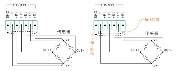
Figure 4.8 6-wire connection method of load cell Figure 4.9 4-wire connection
