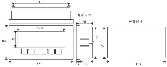
Figure 2.2 installation dimension of display panel
