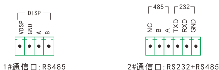
Figure 4.10 schematic diagram of two communication interfaces of instrument
