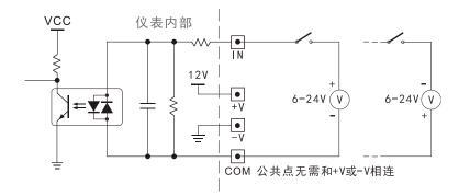
Figure 4.4 Schematic diagram of DC voltage signal input connection 4.2 Connection method of switch output port
