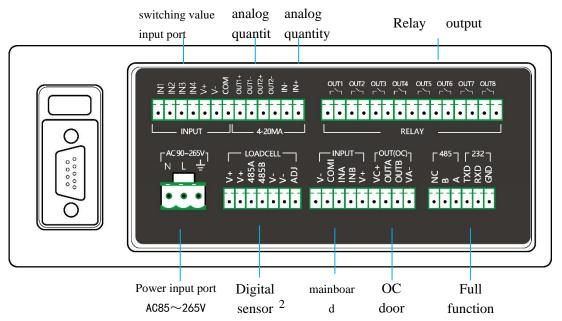
Figure 3.2 Functional Schematic Diagram of B Side of Host Panel Note: Outlet OUTA(OUT9) and OUTB(OUT10) of 1:0C gate are multiplex ports, which can be connected with large screen and stepping motor. Note: Mainboard input port INA corresponds to IN5, INB corresponds to IN6, and high-speed pulse port is common input port corresponding to IN7. IV. Connection method of instrument port
