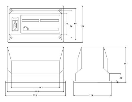
Figure 2.1 Installation Dimensions of Host
