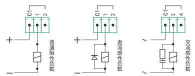
Figure 4.5 Schematic diagram of relay output connection
