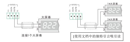
Figure 4.7 Schematic diagram of connection of large screen display Note: Two large screens can also be connected in parallel, for example, the two input lines of two large screens can be connected in parallel in the left figure. **4.4 Connection method of load cell**
