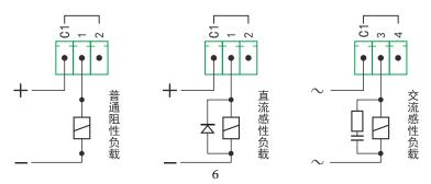
Figure 4.5 Schematic diagram of relay output connection
