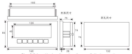
Fig. 2.2 Installation dimension diagram of display panel
