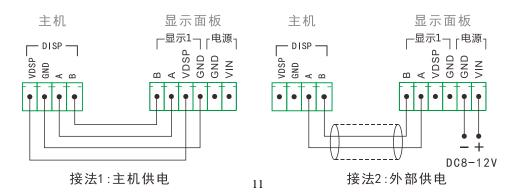
Fig. 4.15 Connection Method between Host and Display Panel
