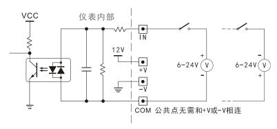
Figure 4.4 Schematic diagram of DC voltage signal input connection
