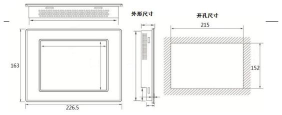
Figure 2.3 Installation Dimensions of Touch Screen
