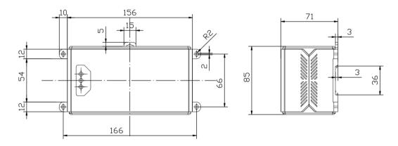
Figure 2.1 Installation Dimensions of Host
