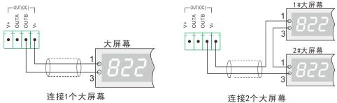
Figure 4.7 Schematic diagram of connection of large screen display
