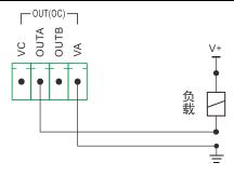
Fig. 4.8 schematic diagram of output connection of npn OC gate
