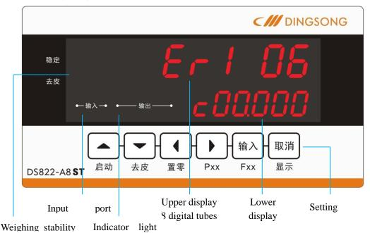
Figure 3.3 Functional diagram of display panel (front)
